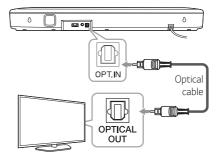
Select the input source to optical by pressing OPTICAL button on the remote control.
