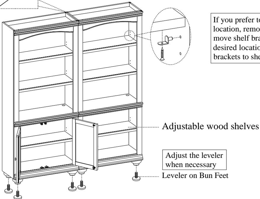
If you prefer to adjust the shelf location, remove the screws and move shelf brackets to the desired location. Then secure the brackets to shelf with screws.
