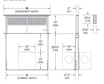
NOTE: Shown with front mounted internal blower with 6" (152) round discharge, dashed line represents rear mount.
