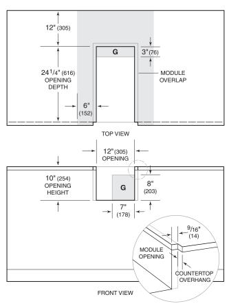
NOTE: Shaded area above countertop indicates minimum clearance to combustible surfaces, combustible materials cannot be located within this area. An insulating liner is not required.
