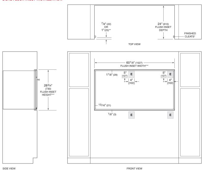
NOTE: Location of electrical supply within opening may require additional cabinet depth. A dual installation kit is required for this installation.
