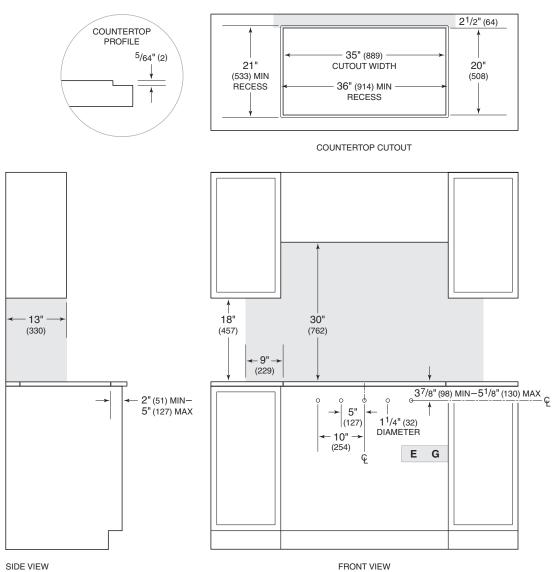
NOTE: Shaded area above countertop indicates minimum clearance to combustible surfaces, combustible materials cannot be located within this area.
