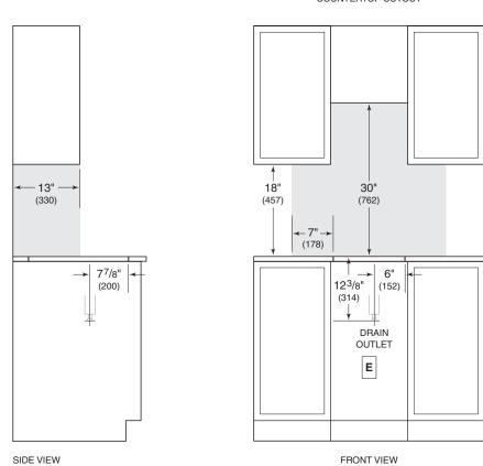
NOTE: Shaded area above countertop indicates minimum clearance to combustible surfaces, combustible materials cannot be located within this area.
