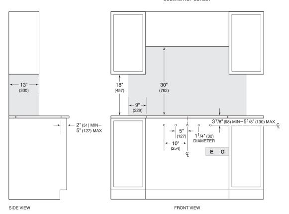
NOTE: Shaded area above countertop indicates minimum clearance to combustible surfaces, combustible materials cannot be located within this area.
