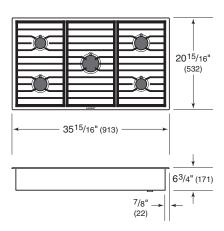
A minimum 2" (51) is required from the bottom of the cooktop to combustible materials. If the cooktop is installed above an oven, a minimum of 1/4" (6) is required between the units.
