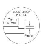
RECESS FOR FLUSH INSTALLATION
