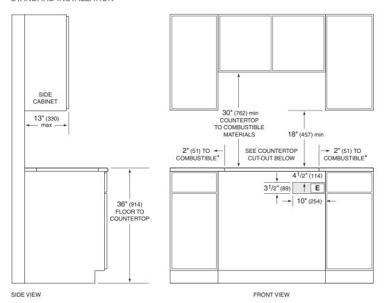
\*Minimum clearance from cooktop cut-out to combustible materials up to 18" (457) above countertop. NOTE: Electrical location applies only to installation with built-in oven.
