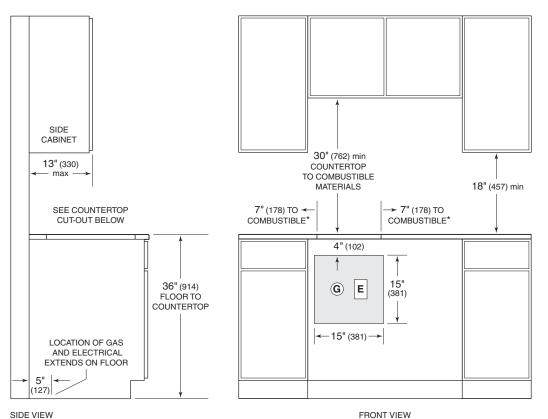
\*Minimum clearance from cooktop cut-out to combustible materials up to 18" (457) above countertop. NOTE: Application shown allows for installation of two 15" (381) modules side by side.
