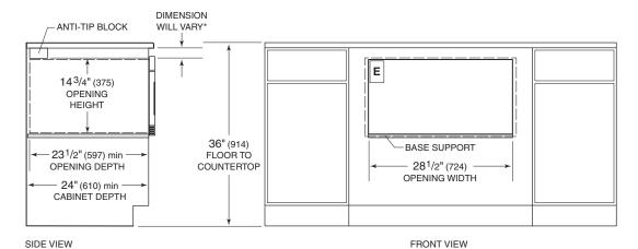
\*Dimension must accommodate height of anti-tip block and drawer face overlap.
