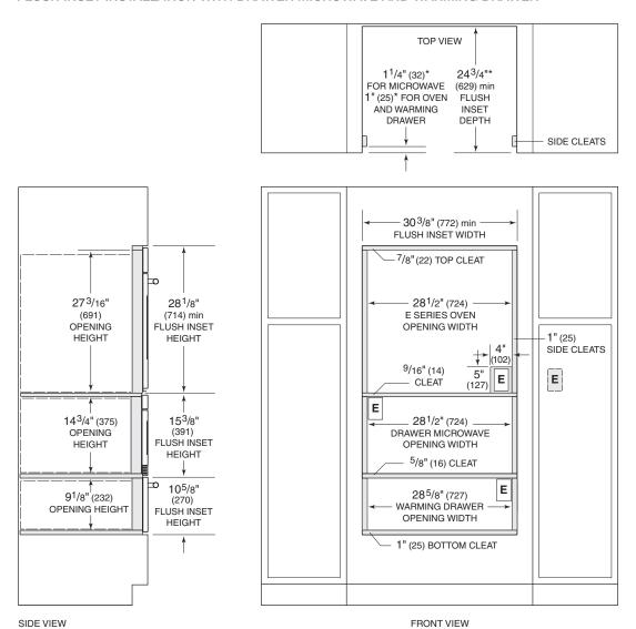
NOTES: Minimum base support for oven 250 lbs (113 kg). Location of electrical supply within oven opening may require additional cabinet depth.
