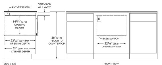
\*Dimension must accommodate height of anti-tip block and drawer face overlap. NOTE: Dashed line represents profile of unit.
