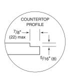
RECESS FOR FLUSH INSTALLATION
