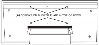
Secure the blower by installing 2 more screws into the locations shown below. Reinstall impeller and cover. Also, reinstall filter support. Plug ventilator's power cord into receptacle inside the hood.
