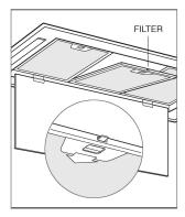
3 Place the charcoal filters on both sides of the blower and rotate the filters counter-clockwise to secure.
