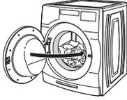
**IMPORTANT:** Push load fully into the washer. Make sure no items are resting on the rubber seal to avoid trapping them between the seal and the door window.
