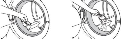
Single-dose laundry packets, Oxi-type boosters, color-safe bleach, or scented crystals can be added to the drum prior to adding laundry. When using single-dose laundry packets, make sure that the bulk dispenser is disabled or off.
