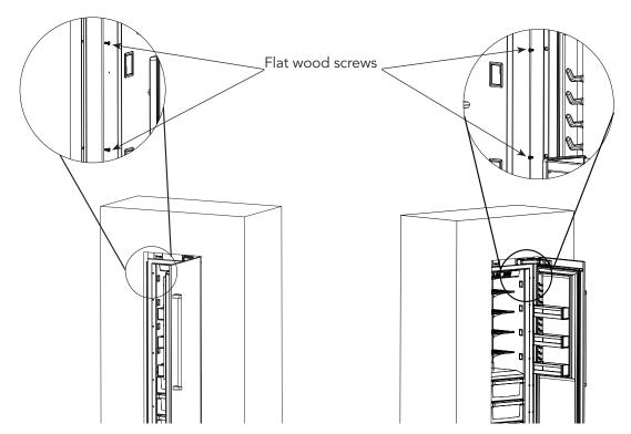
**Door Panel Adjustments** On the side of each panel, at the top and bottom there is a vertical slot with a cam spacer for front to back adjustments. In the center, there is a horizontal adjustment for up and down. All hardware needs to be loosened before adjusting.
