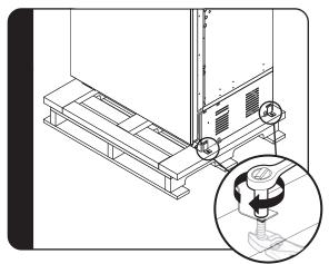
Remove shipping brackets from skid by removing four bolts (two on each side) with a 1/2" (1.3 cm) deep-well socket wench and a pair of pliers. *Note: Tilting unit is not required to remove shipping brackets.*
