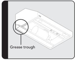
When cleaning filters, always remove the grease trough and clean by soaking in a sink with hot soapy water.
