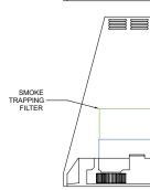
11) Refer to the Air Recovery System Owner and Maintenance Guide for proper hood operation. Test all blower and light functions to ensure they are operating properly.
