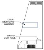
9) Move the canister all the way to the back and then lower the canister over the blower discharge. Shift the canister front to back and left to right to make sure that the blower discharge and canister have fully engaged.
