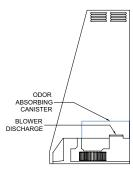
10) With the gasket side facing down, nest the smoke trapping filter element into the pocket that forms the top of the odor absorbing canister. The filter may have a rectangular base so rotate as necessary. Replace the enclosure removable panel.
