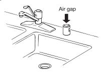
Use <sup>1</sup>/<sub>2</sub>" minimum I.D. drain line fittings.
