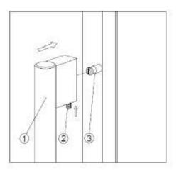
Locate the handle(1)over the pins(3)of the door and tighten the
