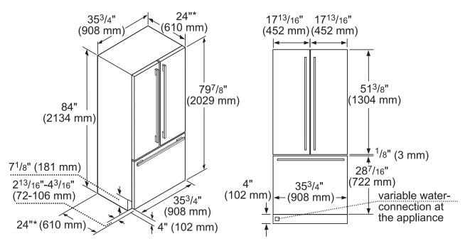
\*Excludes thickness of door panel. If standard panel with <sup>3</sup>/4" thickness is mounted, total depth is 24 <sup>3</sup>/4".
