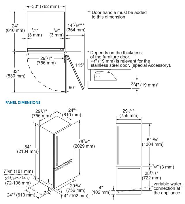
\*Excludes thickness of door panel. If standard panel with <sup>3</sup>/4" thickness is mounted, total depth is 24 <sup>3</sup>/4".
