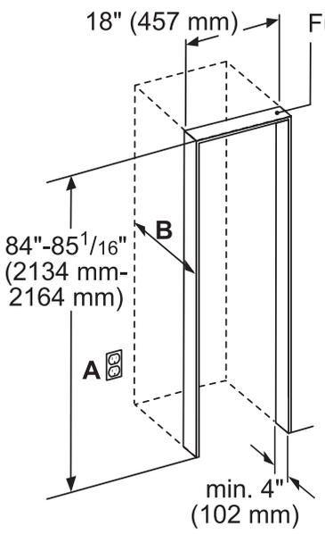
**A:** Area for installation of power connection.
