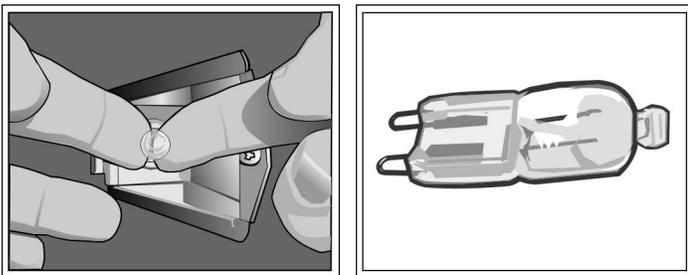
8. Replace the halogen bulb. Grasp the new bulb with a clean, dry cloth. Align the bulb prongs with the socket holes and press into place. Direct finger contact with the bulb may cause premature bulb failure.
