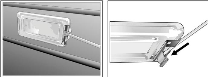
5. (A) Push the screwdriver blade inward to disengage the catch from the slot in the light housing. Support the glass lens cover to prevent it from falling.
