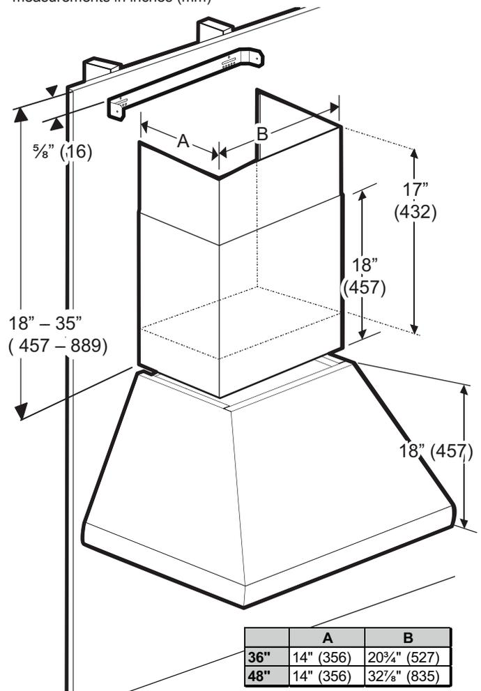
3. At the wall stud locations, measure 5/8" (16 mm) down from the ceiling to the top of the bracket.
