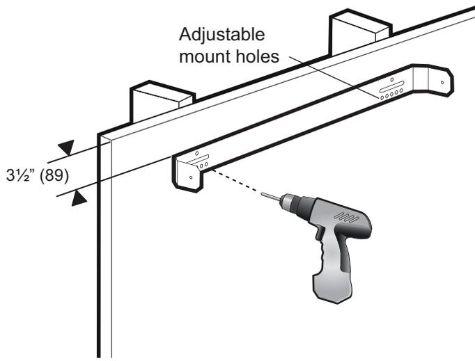
7. Carefully pull the top part of the extension upwards. Screw the left and right sides of the extension to the mounting bracket with the supplied stainless screws.
