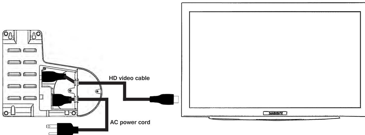
Connect the included 15-foot HD cable to the HD jack on the underside of the receiver. Connect the other end to one of the HD inputs on the TV. Turn on the TV and select the HD input you used to connect the receiver.
