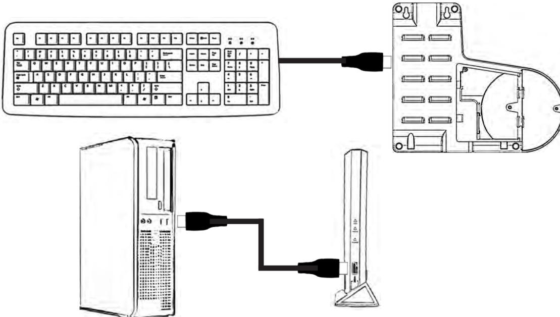
Now use a female-to-female USB cable to connect the USB jack on the transmitter to any USB input on the computer. The USB device connected to the transmitter should now be able to operate the connected computer through the wireless link.
