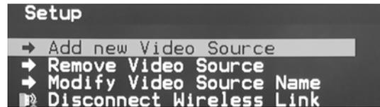
Use the up/down cursor keys on the remote to highlight "Add New Video Source" on the menu, then press the OK button at the center of the cursor keys. You will see a message on-screen that says "Please Activate Registration on Transmitter Unit." Now push the reset button on the transmitter.
