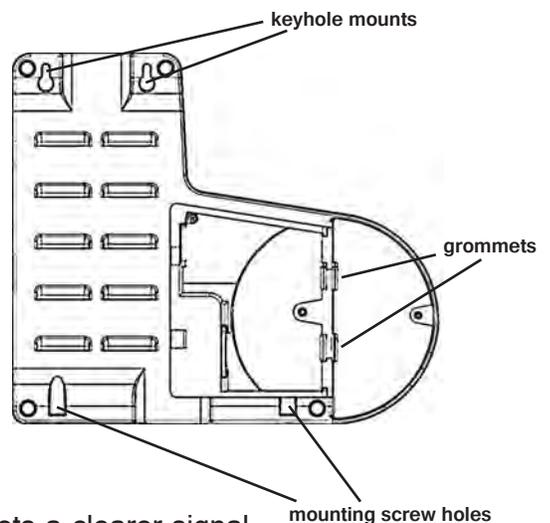
You have two mounting options for the receiver. You can attach it directly to a vertical surface using the keyhole mounts, with two wood screws spaced 2-1/4 inches apart, and installed so that the heads are 1/4-inch above the surface. Or you can attach the receiver directly to a horizontal surface using the mounting screw holes on the bottom.
