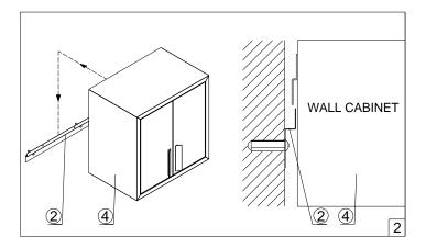
To secure the cabinet to the mounting bracket, use the two supplied screws (5).
