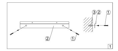
**NOTE:** Using all of the holes in the mounting bracket will ensure the most stable mounting for the cabinet.
