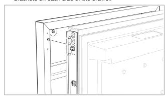
16 Install and secure the remaining screws through the brackets and into the panels.
