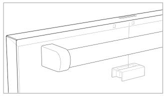
13 Install the lock assembly on the upper panel, then use the key to verify the cam rotates downward.
