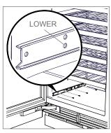
Disassemble slide assembly
