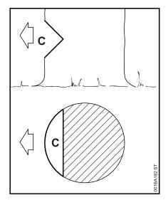
Felling notch (C) – determines the direction of the fall
