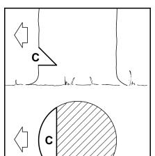
Felling notch (C) – determines the direction of the fall
