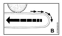
Pushback occurs when the saw chain on the top of the bar is suddenly stopped when it is pinched, caught or encounters a foreign object in the wood. The reaction of the saw chain may drive the chain saw rapidly straight back toward the operator and may cause loss of chain saw control, which, in turn, may cause serious or fatal injury. Pushback frequently occurs when the top of the bar is used for cutting.
