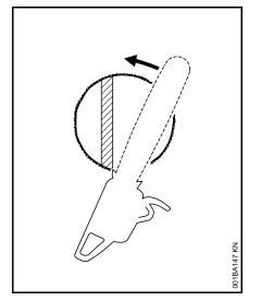
Engage the bumper spikes of the chain saw directly behind the location of the intended hinge and pivot the saw around this point only as far as the hinge. The bumper spike rolls against the trunk.
