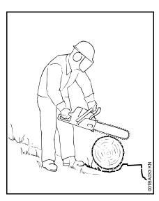
Bucking is cutting a log into sections.
