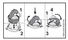
An improperly tightened fuel filler cap can loosen or come off and spill quantities of fuel. To reduce the risk of fuel spillage and fire from an improperly installed fuel cap, correctly position and tighten the cap in the fuel tank opening:
