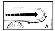
Pull-in occurs when the saw chain on the bottom of the bar is suddenly stopped when it is pinched, caught or encounters a foreign object in the wood. The reaction of the saw chain pulls the chain saw forward and may cause the operator to lose control.
