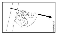
Position the chain saw in such a way that your body is clear of the cutting attachment whenever the engine is running. Stand to the left of cut while bucking. Never put pressure on the chain saw when reaching the end of a cut. The pressure may cause the bar and rotating saw chain to pop out of the cut or kerf, go out of control and strike the operator or some other object. If the rotating saw chain strikes some other object, a reactive force may cause the moving saw chain to strike the operator.
