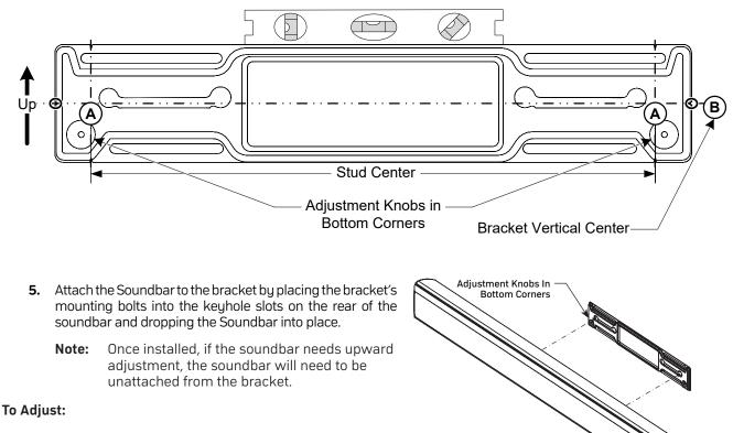
Remove the soundbar from the bracket, then adjust the thumbscrews on the bracket by hand or using a flathead screwdriver if necessary.
