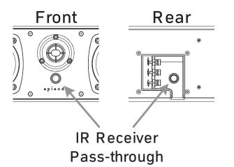
To maintain accurate IR reception, a spacer has been included to allow for the front edge of the IR receiver to be flush with the back of the grille cloth. This will ensure that IR reception is at its maximum level.
