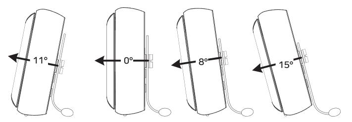
After installing the kickstand and placing the Soundbar, adjust the angle of the speakers towards the listener's ears. If the speakers point away from the listener's ears, slide the kickstand up or down to achieve the proper angle. Note that the kickstand can be inverted when the Soundbar is pointing down.
