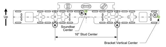
**5.** Attach the Soundbar to the bracket by placing the bracket's mounting bolts into the keyhole slots on the rear of the soundbar and dropping the Soundbar into place.
