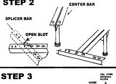
inserting the rivet at the end of the center support bar into the center keyhole slot of the slpicer bar, then slipping the open slot on the splicer bar under the rivets on the center bar and swing into place.
