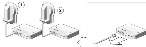
Both sensors plug into a single common processor
