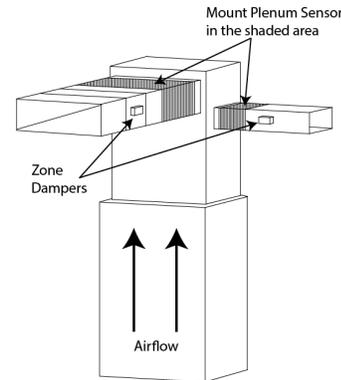
2. In the area selected, drill a 5/8 inch hole into the ductwork.
