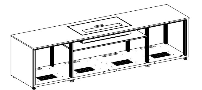
Model LG HU86LA 90" Diagonal image: 2.2" from back of projector to front of screen
