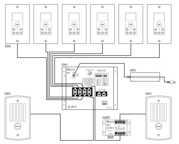
Six-zone ComPoint system with Advanced Keypads and an optional Door Strike Release Module
