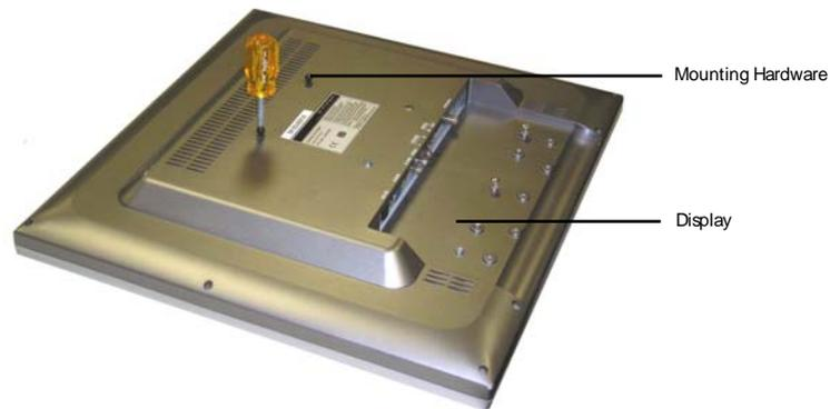
3. Lift the display and carefully guide the display with the two screws into the keyhole openings.
