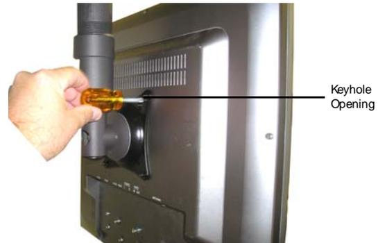
4. Let the display rest in this position while you insert the lower mounting screws.
