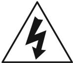
The graphic symbol of a lightning flash with an arrow point within a triangle signifies that there is dangerous voltage within the unit and it poses a hazard to anyone removing the cover to gain access to the interior of the unit. Only qualified service personnel should make any such attempt.
