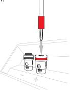
**Banana Plug Connection** Remove binding post plugs and insert the banana plug into the top of the binding post.
