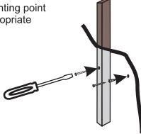
VIII. For the Imagine W1, line up each mounting screw on the wall-mounting bracket with the keyhole slots on the speaker, and let the speaker slide straight down, allowing each screw head to slide-and-lock into the slot for a secure mount.
