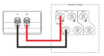
**Observe Proper Connection Polarity**
