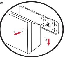
IX. For the Imagine W3, fit the speaker's contoured groove into the mounting edge of the bracket.
