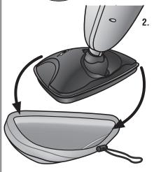
Remove the Microfiber Cleaning Pad over the floor head.
