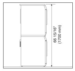
The Miele washing machine can be installed as part of a washer-dryer stack in combination with a Miele tumble dryer. An appropriate stacking kit\* is required.
