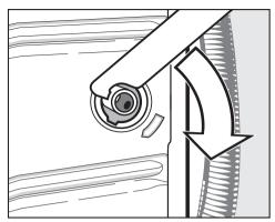
Turn the right shipping strut clockwise 90° with the enclosed combination wrench.
