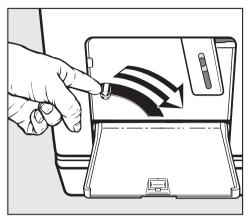
Press the lever for the emergency drain down and hold until you hear no more water running out.
