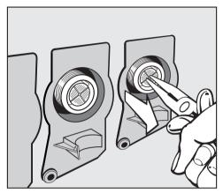
Using needle nose pliers, remove the plastic filter by pulling on the bar (see illustration). Rinse under running water and return. Replace the filter and seal, then reconnect the hose.
