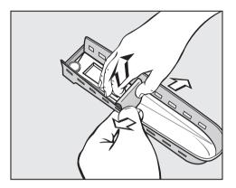
Push the insert apart and remove the siphon for easy cleaning.
