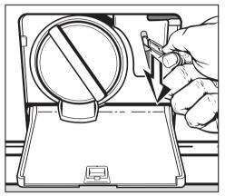
Insert a screwdriver into the notch, beside the lint trap, pull it down. The door will now open.
