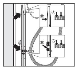
Fasten the shipping struts at the rear side of the washer. Take care to insert the drill holes, (B), into the clamps, (A). Movement of the washer without the shipping struts in place should be kept to a minimum. The shipping struts should be stored on the back of the washer for future use. They must be reinstalled before moving the machine.
