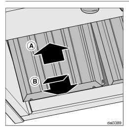
■ Reinsert the baffle filters by pushing the filter upwards (a) then pushing it in (B).
