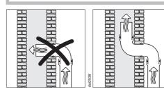
■ If the exhaust air is to be ducted into a flue, the duct must be directed in the flow direction of the flue.
