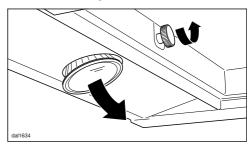
Turn the bolt counterclockwise as far as it will go. The halogen lamp will then drop down towards you.
