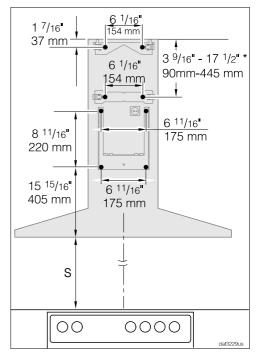
When installing a custom back wall with pre-drilled holes, please refer to the drilling distances in the drawing above (screws Ø <sup>3</sup>/<sub>16</sub>" (5 mm)).
