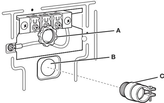
Unscrew the removable conduit connector (A) and any screws from a 3/4" (19 mm) UL listed strain relief (UL marking on strain relief). Put the threaded section of the strain relief (C) through the hole below the terminal block opening (B). Reaching inside the terminal block opening, screw the removable conduit connector (A) onto the strain relief threads.
