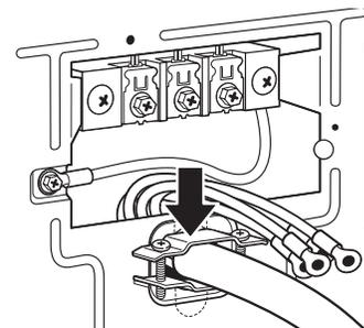
Put power supply cord through the strain relief. Be sure that the wire insulation on the power supply cord is inside the strain relief. The strain relief should have a tight fit with the dryer cabinet and be in a horizontal position. Do not further tighten strain relief screws at this point.
