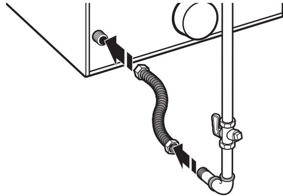
**NOTE:** Do not kink or damage the flexible stainless steel gas line when moving the dryer.
