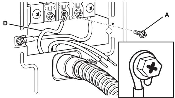
3. Place hooked ends of remaining direct wire cables (hooks facing right). Squeeze hooded ends together and tighten outer terminal block screws (F). Finally, re-install terminal block cover and tighten hold-down screw. Go to "Complete Installation" section.
