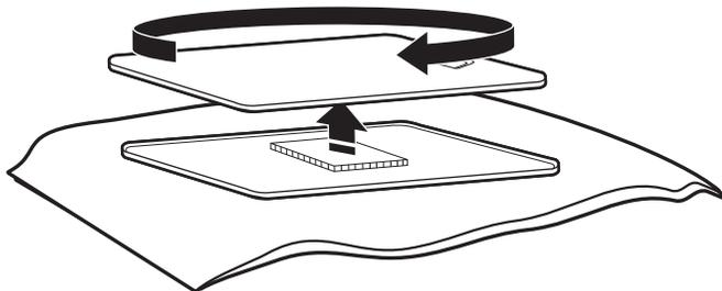
7. Be certain to keep cardboard spacer centered between doors. Reattach outer door panel to inner door so handle is on the side where hinges were just removed.
