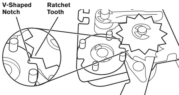
4. Insert a narrow, flat-blade screwdriver under the timing cam near the clock shaft. Gently lift cam straight up and off shaft, making sure that the V-shaped notch clears the ratchet tooth.
