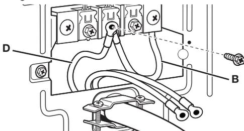
3. Connect remaining wires under outer terminal block. Tighten screws (F).
