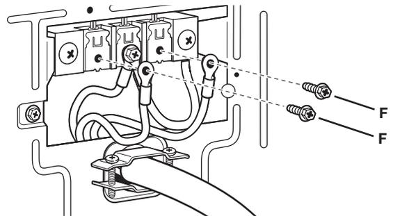
4. Connect a separate copper ground wire (G) under the external ground conductor to screw (C) an adequate ground. Finally, re-install terminal block cover and tighten hold-down screw. Go to "Complete Installation" section.
