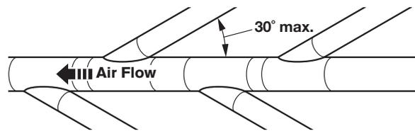
The maximum angle of each vent entering the main vent should not be more than 30°.
