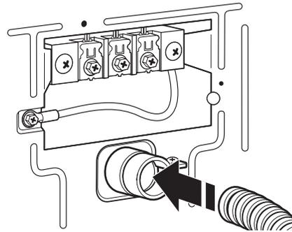
Put direct wire cable through the strain relief. The strain relief should have a tight fit with the dryer cabinet and be in a horizontal position. Tighten strain relief screw against the direct wire cable.
