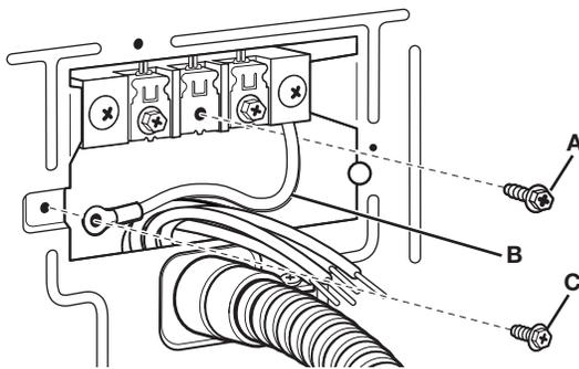
2. Connect neutral ground (B) and place hooked end (hook facing right) of neutral wire (white or center wire) cable (D) under center terminal block screw (B). Squeeze hooked end together. Tighten screw.
