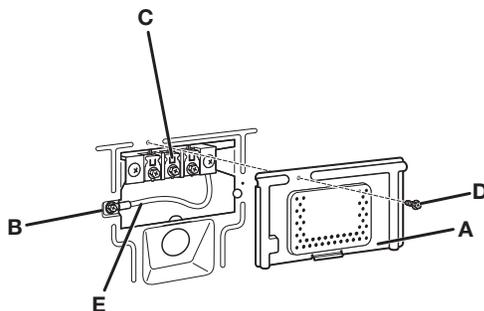
Before you start, disconnect power. Remove hold-down screw (D) and terminal block cover (A).
