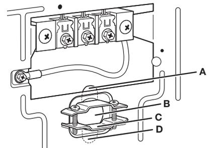
Remove the screws from a 3/4" (19 mm) UL listed strain relief (UL marking on strain relief). Put the tabs of the two clamp sections (C) into the hole below the terminal block opening (B) so that one tab is pointing up (A) and the other is pointing down (D), and hold in place. Tighten strain relief screws just enough to hold the two clamp sections (C) together.
