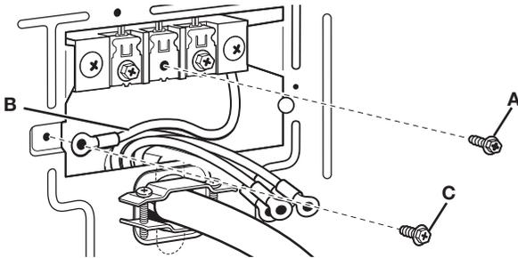
2. Connect neutral ground (B) and neutral wire (white or center) (D) to center terminal block. Tighten screw.
