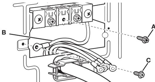
2. Connect neutral ground wire (B) and neutral wire (white or center) (D) of power supply cord/cable under center terminal block. Tighten screw.
