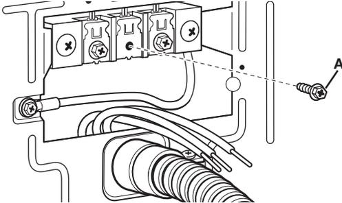
2. Place hooked end (hook facing right) of neutral wire (white or center wire) (D) cable under center terminal block screw (A). Squeeze hooked end together. Tighten screw.
