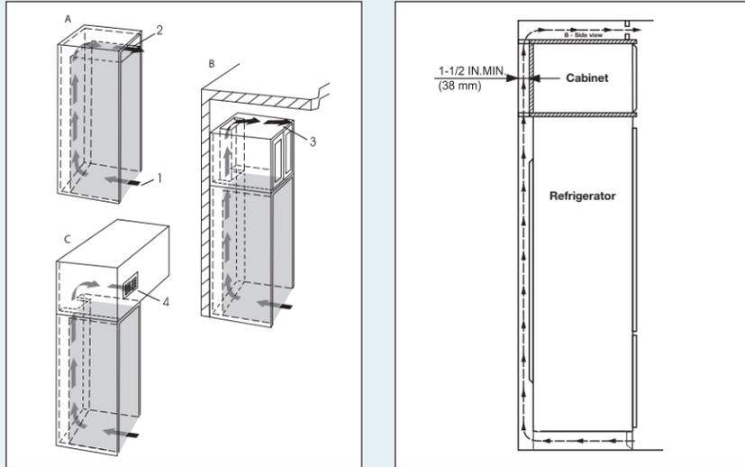
This type of cabinet must be carefully constructed using the correct dimensions and it must provide suitable ventilation to ensure proper appliance operation.
