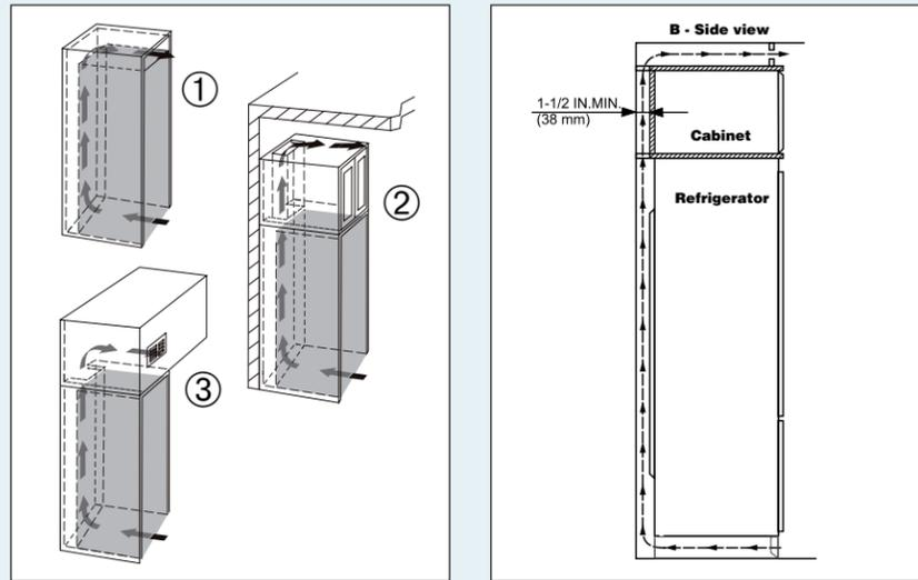
Do not restrict the air flow. The opening can either be directly over the appliance ①, above the cabinet and below the ceiling ② or through a vent installed in a soffit ③.
