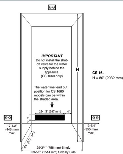
The appliance can be used freestanding or semi built-in. If semi built-in, consider the cabinet opening dimensions.
