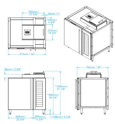
\*overall height adjusts +/-20mm / 3/4" on stainless steel leveling legs
