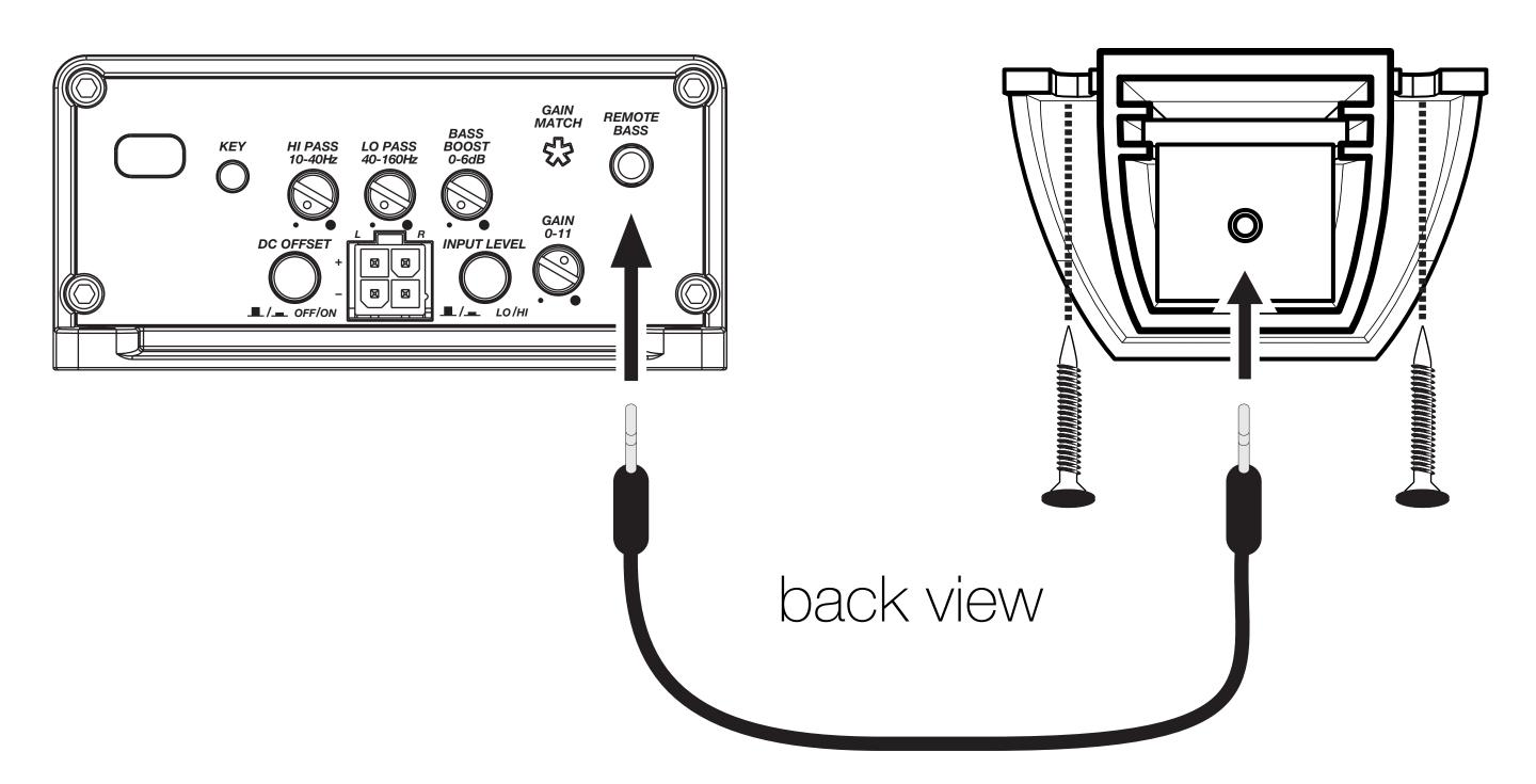
Remote cable passes audio; do not run cable parallel to power wires.
