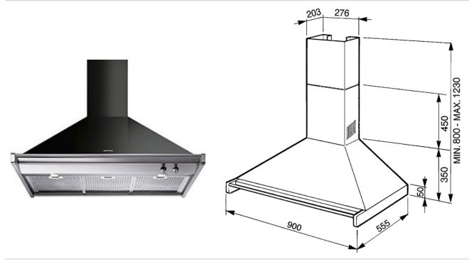
• Exclusive Classic design • Wall mounted ventilation hood • High quality stainless steel • Stylish ergonomic control knobs • Front mounted controls for lights and vent speeds • 1 motor • Vented or recirculating • 4 speeds • 2 halogen lights (2x20W) • 3 dishwasher safe stainless steel grease filters • 600 CFM max. setting • Vent duct size @ 6" • Voltage rating: 120V / 60Hz / 4.5 Amps
