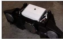
If access to the amplifier is required, remove the four Allen Head screws that secure the top cover.
