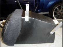
**STEP 5** Place a supplied lock washer, flat washer and mounting bracket onto three of the supplied bolts.
