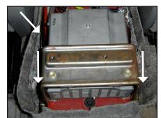
**S T E P 2** Remove the pair of screws that are at the bottom of the storage bucket.
