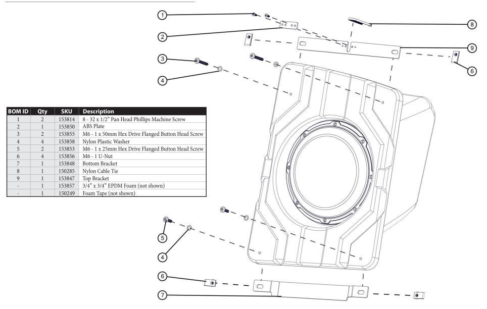
Note: For optimum performance, JL Audio recommends applying the included Foam Strips (or sound damping material) to surrounding plastic panels to reduce unwanted vibrations.
