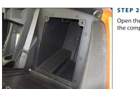
Open the storage compartment, and remove the compartment door.
