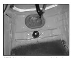
**STEP II:** While second person is holding the Stealthbox into position (inside of vehicle). Place flat washer, lock washer and nut onto the exposed threaded rod and secure.
