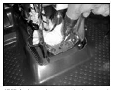
**STEP 6:** Locate the bracket that is mounted to the floor with a pair of bolts. Use the middle non-used hole as a drilling guide.
