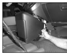
**STEP 3:** Remove the OEM plastic woofer cover, by pulling out plastic push clips that are located on each side.
