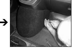
**STEP 13:** Mount the supplied carpeted side panels with the four supplied Phillips screws.
