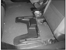
**STEP I:** Remove the front passenger's plastic seat rail cover, located under and rear of the seat. Remove the rear mounting bolts, using a 14mm socket.
