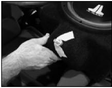
**STEP 8:** Thread in the supplied socket cup set screw into the Stealthbox, leaving about 1 3/4" exposed. Make sure that the slotted end of the threaded rod is exposed. Place the supplied spacer onto socket cup screw.
