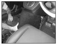
**STEP 10:** Place the Stealthbox into location. Using the socket cup set screw as guide and place through the drilled hole from **STEP 6**.
