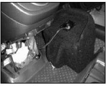
**STEP 9:** Run speaker wire to the Stealthbox location and attach to terminal.
