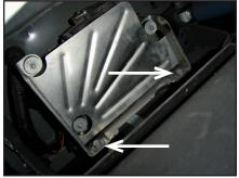
SUVs with the air compressor only. STEP 5 Look up into the passenger's side rear wheel well. You will see this metal plate as in the picture.
