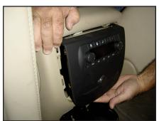
**STEP 8**Pry the rear face to the rear of the vehicle.
