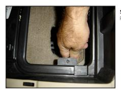
**STEP 6**Pull the wiring harness off the tab.
