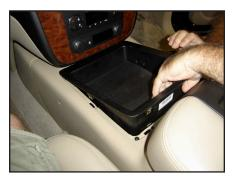
**S T E P 4**Remove the cup holders from center console by pulling upwards.
