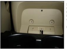
**S T E P 1 0**From the back side of the center console, fold down the cup holders.
