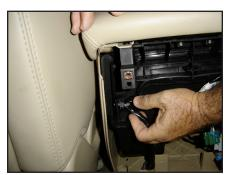
Remove the wiring harness that is secured to the driver's side of the center console.
