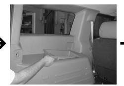
**STEP 5:** By pulling up, remove the driver's side rear storage bucket.
