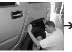
**STEP 17:** Mount the plastic inner wheel well and plastic trim from **STEPS 6 & 7**.
