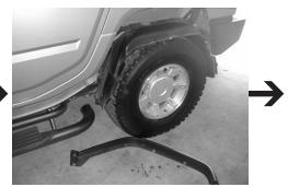
**STEP 8:** Rest the plastic inner wheel well on the rear tire. Keep the trim and all the mounting hardware together.
