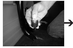
**STEP 19:** With the spare tire rack placed into position. Loosely tighten the lower factory bolts to the lower mounting feet.
