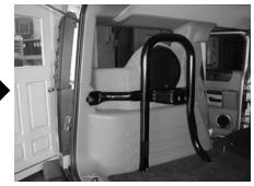
**STEP 22:** With the spare tire rack properly positioned, it should not interfere with the enclosure.
