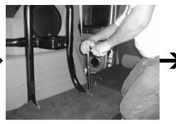
**STEP 21:** Align the spare tire rack, for proper positioning.
