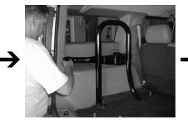
**STEP 4:** With an 8mm socket, remove the four bolts that secure the spare tire rack.
