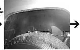
**STEP 7:** With the plastic trim out of the way, remove the plastic inner wheel well.
