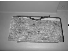
**STEP 9: (Inside the vehicle)** Cut and remove the factory jute(sound deadening), from the removed storage area, from **STEP 5**.
