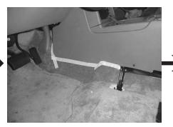
**STEP 7:** Once the front seats have been removed, you will need to outline the outside of the center console with masking tape(not supplied). This will help in future steps.
