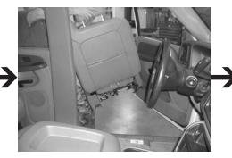
**STEP 6:** To remove the front bucket seats, you use a 15mm socket(not supplied) for the front nuts and a 12mm(not supplied) for the rear bolts.
