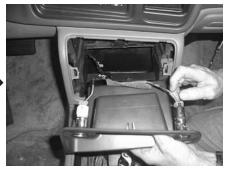
**STEP 8:** With the upper storage pocket panel removed. You can view a pair of bolts. Using a 10mm socket(not supplied), remove these bolts.
