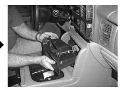
**STEP 2:** Moving down to the top portion of the center console. Pull the upper storage pocket panel out and disconnect the electrical outlets.
