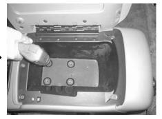
**STEP 5:** To remove the main storage bucket, remove the rubber mat. This will expose the four screws that need to be removed.
