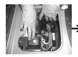
**STEP 9:** Look down in the console from the cup holder area. You need to locate and disconnect a white connection plug. Pull the lever on this white connection plug to disconnect from the wire harness..
