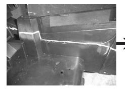
**STEP 32:** The mark line needs to come around this leg. Go down to the inner edge of this flat lip.
