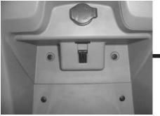
**STEP 21:** With the OEM console out of the vehicle. You need to remove the outside cosmetic console from the inside structure support console.
