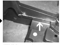
**STEP 27:** This is a view of the driver's side, rear area. The mark lines needs to follow the inner edge of this flat lip.
