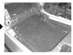
**STEP 43:** When the OEM console is place over the Stealthbox. It should be snug.
