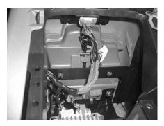
**STEP 46:** Reconnect the rear stereo controls and I2v plug from **STEP 22**.
