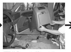
**STEP 10:** To remove the OEM console, lift up on the rear of the console and pull it back away from the dash.
