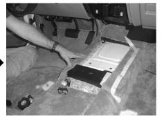
**STEP 19:** With the wire harness properly tucked under the carpet, use double sided tape(not supplied) to secure the carpet to the metal floor.
