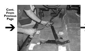
**STEP 12:** Remove the OEM wire harness from the plastic track. Wrap the OEM wiring in black tape.
