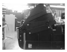
**STEP 23:** To remove the OEM woofer enclosure. Start by drilling out these pair of rivets. Located on the driver side of the console.
