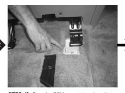
**STEP 42:** Place the OEM console into the vehicle. Sleave the OEM console over the Stealthbox. Make sure that the OEM consoles mounting legs are placed back over the OEM position studs.
