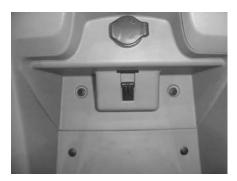
**STEP 47:** Replace the rear of the outer cosmetic console and the four mounting screws from **STEP 21**.
