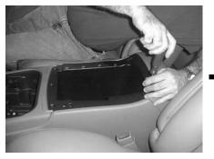
**STEP 4:** On the upper lip of the main storage bucket, remove all the screws, including the storage lid's screws.
