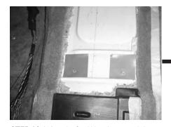
**STEP 16:** When the Stealthbox is removed, the wax square should have the impressions of the socket cup set screws.
