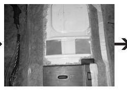
**STEP 14:** With the OEM carpet and the jute(sound deadening) cut out. Position the supplied pair of 3"x3" wax squares in place.
