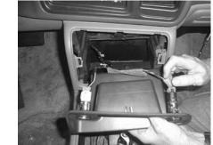
**STEP 45:** With the upper storage pocket in hand from **STEP 4**, reconnect the 12v outlets. Then snap the upper storage pocket back into place.
