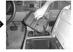
**STEP 3:** Pull the cup holders up and out of the center console.
