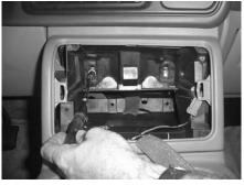
**STEP 44:** The pair of 10mm bolts that where removed in **STEP 5**, need to be replaced. You may have to reposition the OEM console, to have it line up like factory.
