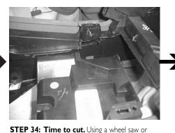
blade saw will be easier to use, then a jig saw. Follow the mark lines with the cutting tool. This is the view of the driver's side, from **STEP 27**.
