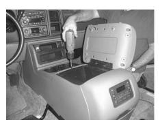
**STEP 48:** Replace the main storage bucket and storage lid from **STEP 6 & 7**.
