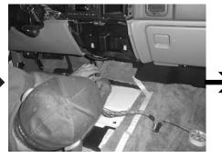
**STEP 18:** The wire harness from **STEP 12** needs to be rerouted over to the other side of the structure support bar under the dash.
