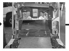
**STEP 41: Time to cut.** Follow the mark lines with the cutting tool.
