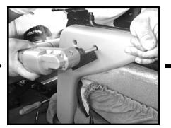
**STEP 2:** Remove the side plastic panel from armrest assembly.
