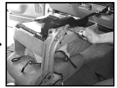
**STEP 4:** Remove the center seat from the armrest assembly, by removing the OEM bolts.
