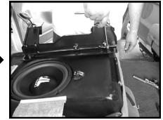
Be sure that the side OEM uphostry flaps are tucked between the seat bracket and the Stealthbox.
