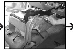
**STEP 10:** With the OEM uphostry applied. Using the supplied 3/8" hex head bolts, mount the armrest assembly to the Stealthbox<sup>™</sup>.
