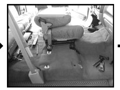
**STEP I3:** Bolt the 40/20/40 split front bench seat back into the truck using the OEM bolts, from **STEP I**.
