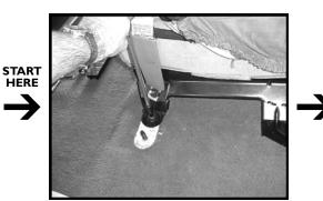
**Step I:** Remove the 40/20/40 split front bench seat from truck.
