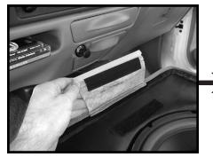
**STEP 9:** Wrap the Stealthbox<sup>™</sup> using the OEM uphostry that was removed in **STEP5**.
